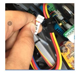
There has 2 cable of z axis ,check those 2 cables , better use multimeter to check connection of very wire of those 2 cables what is mark 'M-PT-Z'
