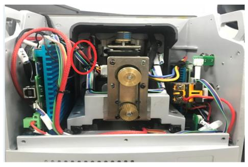
Psl check those position where has cable tie ,to see if has some damage of those cables ,especially for Z , fix it if has any problem
